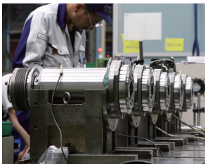
Test running under strict temperature control
