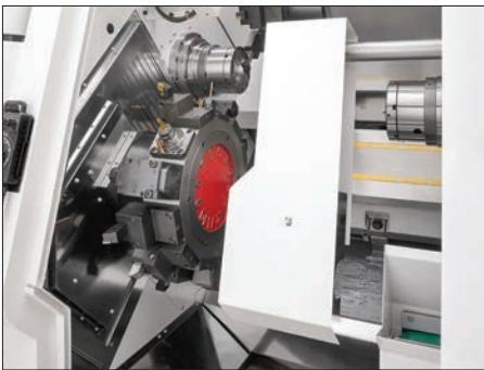
Part catcher (Standard) Discharges workpiece on to conveyor.
